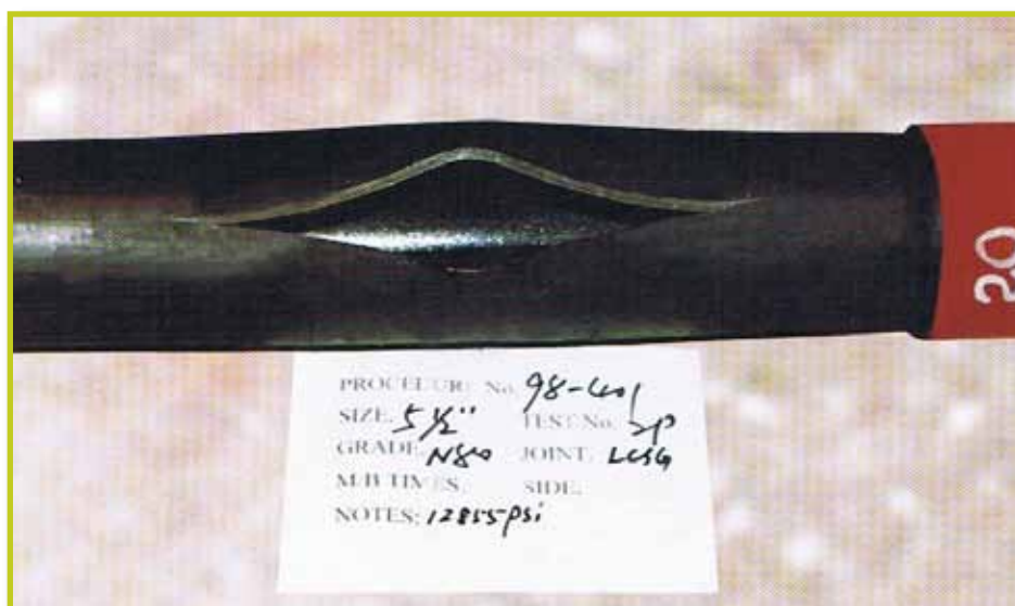
Petroleum Casing Blow Test
